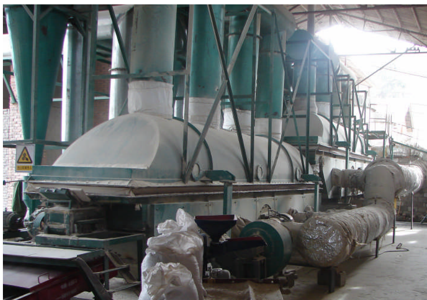
Figure 2. Dewatering and drying process during Phoslock ® manufacturing at Kunming factory, China.
