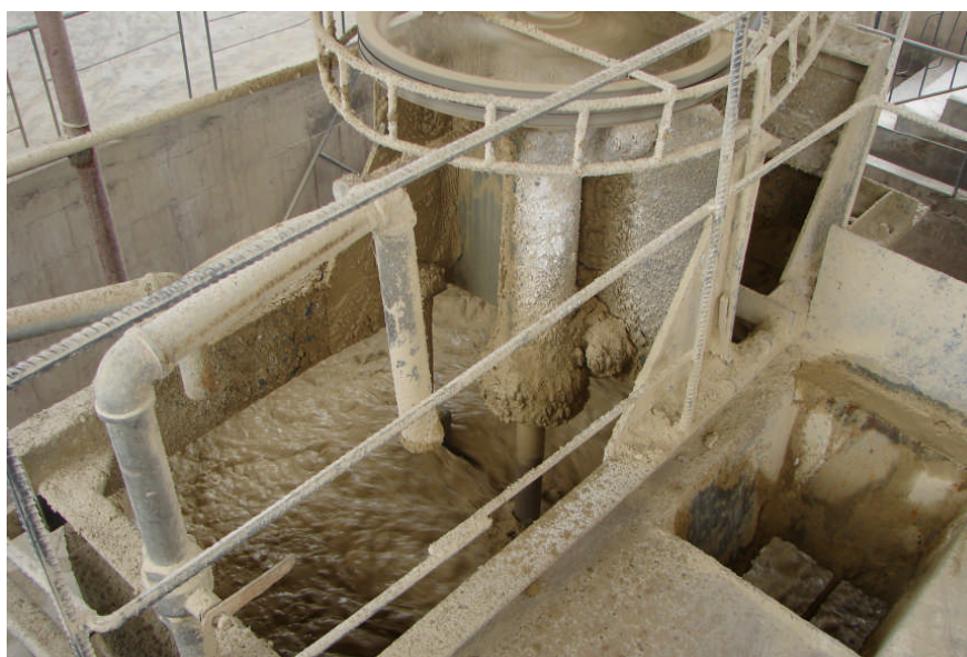
Figure 1. Mixing bentonite clay and lanthanum chloride at Phoslock ® manufacturing factory in Kunming, China.
