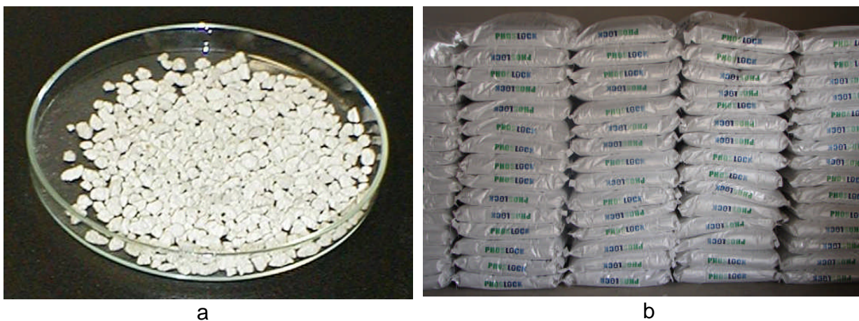
Figure 4. a) Dry, free flowing granular Phoslock ® (2 – 4 mm), b) 25 kg Phoslock ® bag.
